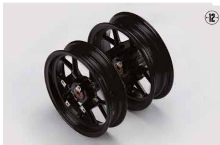
KIT ROUE YCF 12" (2.15 X 12" AVANT/ 2.75 X 12" ARRIÈRE) YCF WHEEL SET 12" (2.15 X 12" FRONT/ 2.75 X 12" REAR)
